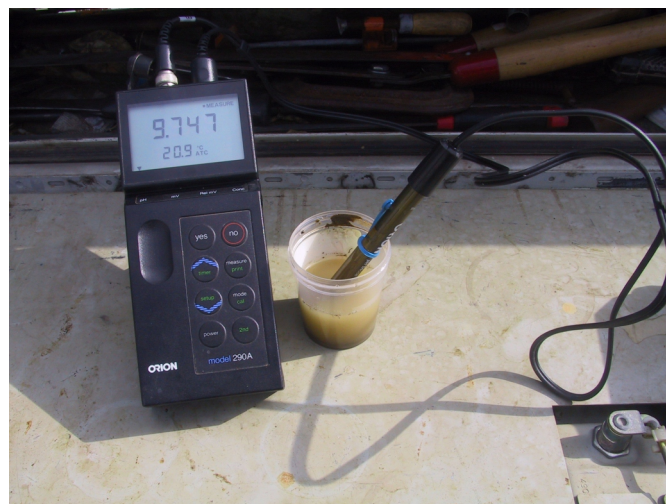
Figure 4.4.3 Portable meters like the one shown here are invaluable for on-the-spot soil chemical properties determination, including pH.
