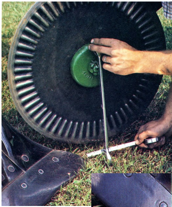
Figure 11 (left). Adjusted fore-and-aft coulters position. Photo: John Deere Service Publ. (1976).
