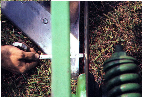
Figure 12 (below). Adjusted horizontal coulters position. Photo: John Deere Service Publ. (1976).
