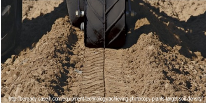
Figure 6 Planter press wheel ensures favorable seed-soil contact by firming the soil 360 degrees around the seed after it is placed in the slit opening. Target soil density of \sim 1.3 \text{ g/cm}^3 surrounding the seed provides optimal movement of nutrients, water, and air through the soil. Source: CaseIH.com
