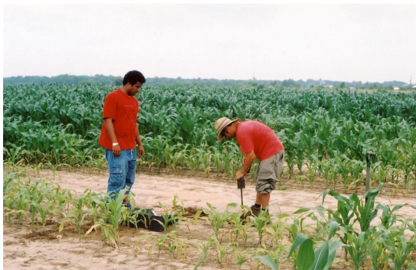
Figure 5. Interns learned to measure soil bulk density and interpret the results. Information derived from bulk density provides insight about the physical condition of the soil with respect to entry and transfer of air, moisture, and heat.
