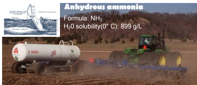
Figure 9. Anhydrous ammonia application rig. Because anhydrous ammonia is a gas at normal atmospheric temperature and pressure, it is stored as a liquid under \sim 1.4 MPa pressure (about 200 psi) and applied via trailing 'nurse' tanks equipped with special valves, hoses, and fittings. Inset: close-up of an anhydrous applicator chisel or 'knife' shank showing injection of anhydrous ammonia gas into soil slit. Photo by Todd Nelson, University of Wisconsin; inset image from Crops and Soils magazine.
