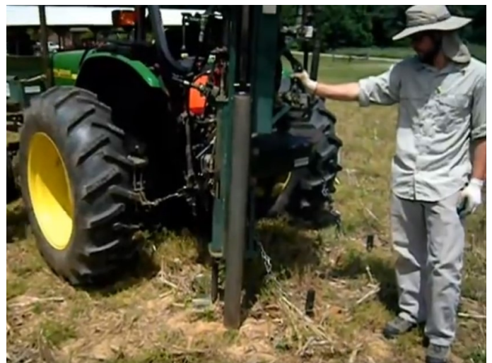
Thin-walled steel Shelby tubes can be attached directly to a machine. This yields a "quasi" or nearly undisturbed core sample suitable for classification and testing.
