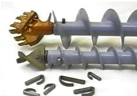
Toothed and fishtail cutter heads attached to solid flight auger stem.
