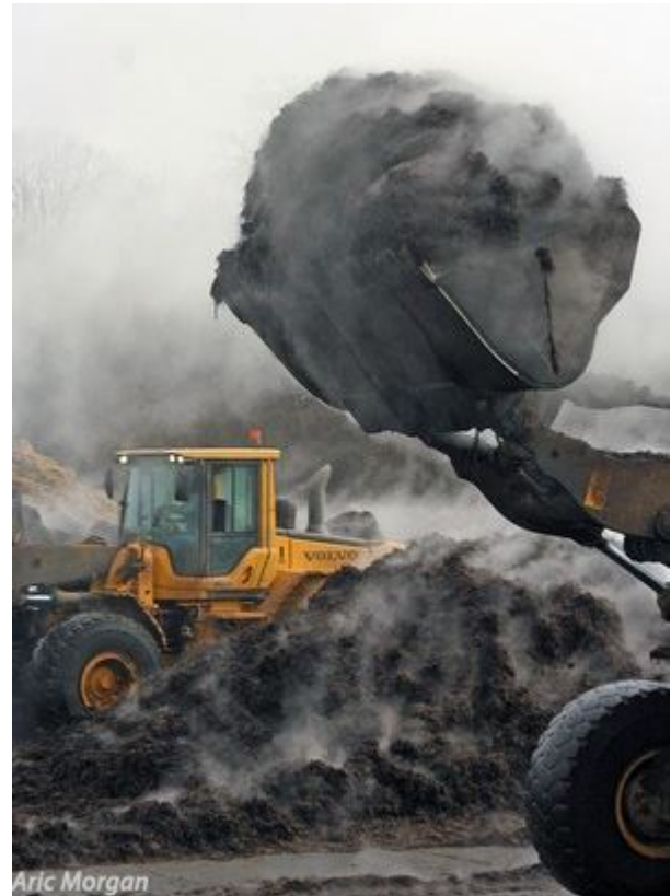
Figure 2. Bucket loaders mix and turn compost in volume. Bulk density is used to convert compost weight ratios to volume ratios for efficient handling.
