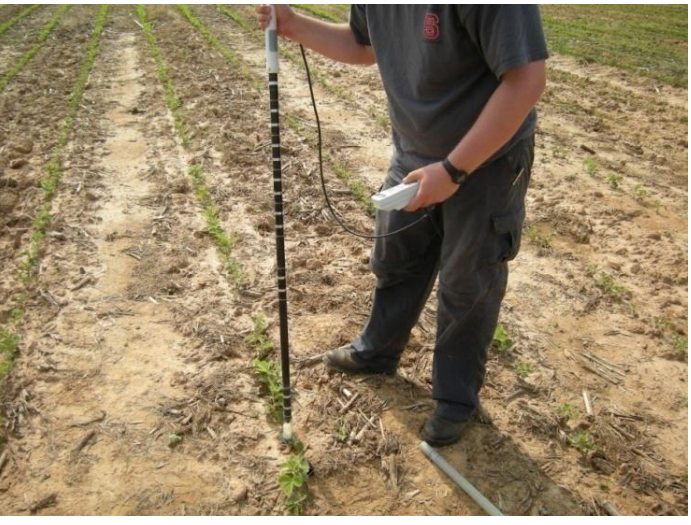
Monitoring profile moisture content in soybean with the PR2/6 capacitance probe. The probe is inserted into a 2.5-cm diameter plastic access tube (above) during measurement.
