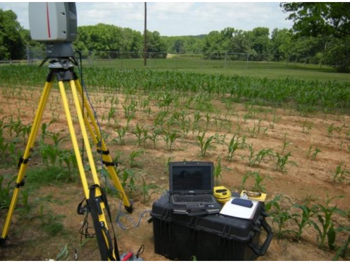
Remote sensing deployed to assess soil surface and profile characteristics: scanning lidar (above) for topography, ground penetrating radar (GPR) and electromagnetic induction measurement of soil electrical conductivity for profile characteristics, and aerial L-Band radar for surficial soil moisture.
