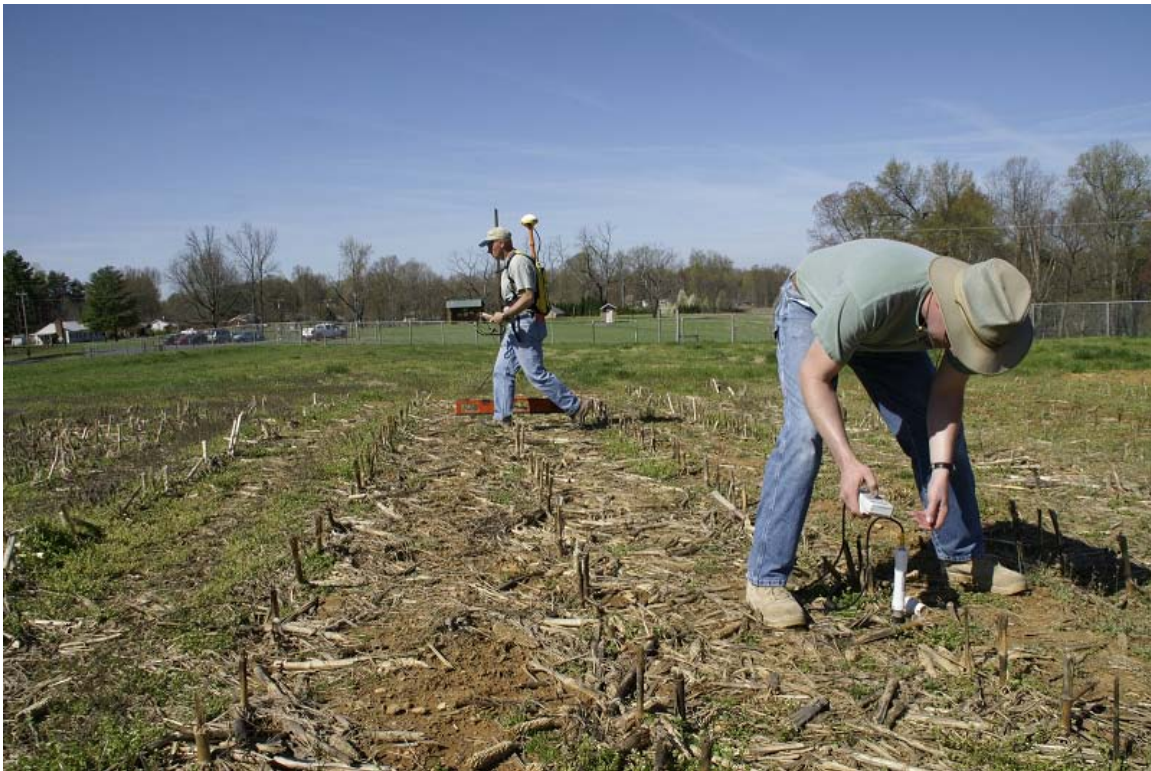
Photo 3. Soil moisture measurements are being recorded in the foreground as an electromagnetic induction (EMI) survey is being conducted in the background with a Geonics EM38 meter at site 1. The test sites were located at the Upper Piedmont Experiment Station near Reidsville, NC.
