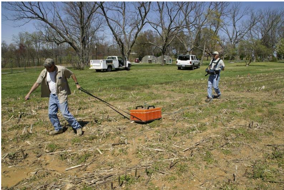
Photo 4. A GPR survey is being conducted with a 200 MHz antenna across an area of Casville soils at site 1. GPR was used to determine depths to contrasting subsurface features such as bedrock and saprolite.
