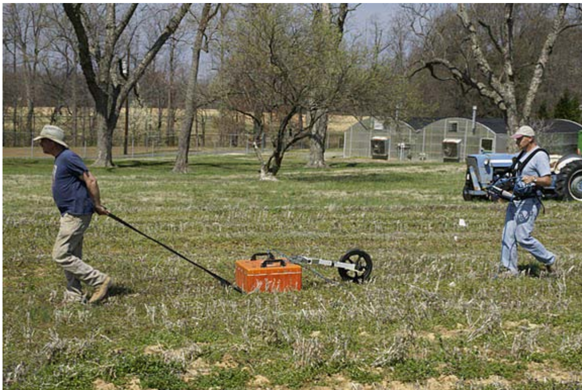
Photo 2. GPR surveys were conducted with the 200 MHz antenna across the sites. GPR was used to determine depths to contrasting subsurface features including bedrock, saprolite and buried utility lines.
