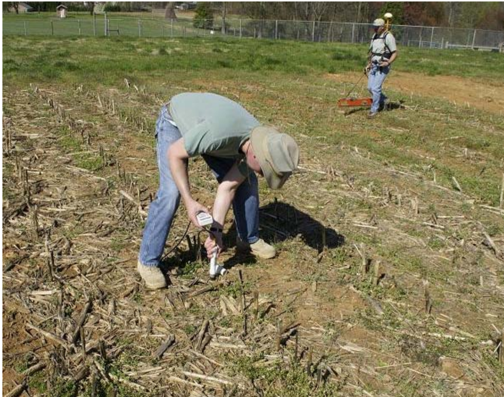
Photo 1. Soil moisture measurements are being recorded in the foreground as an electromagnetic induction (EMI) survey is being conducted in the background at the Upper Piedmont Experiment Station located near Reidsville, NC.
