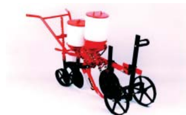
PLATE 66 Latest version of direct-sowing machinery for animal traction produced in Mafra municipality.
