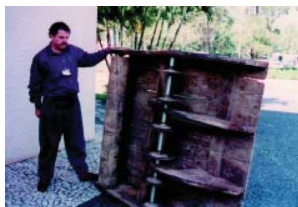
PLATE 80 Roller with discs developed by small farmers in the Alto Vale de Itajaí region
