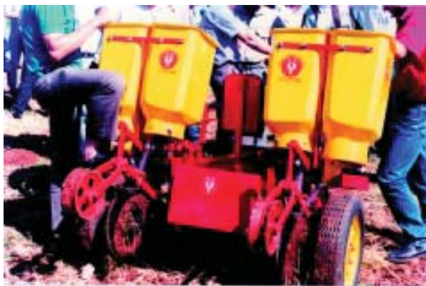
Plate 72 Two-row direct-sowing and fertilizing equipment with tired wheels from Rio Grande do Sul. View from the rear
