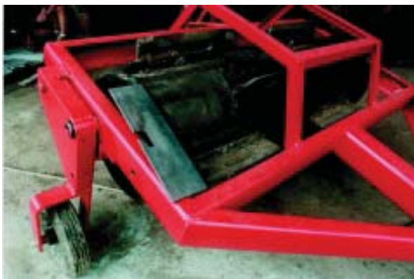
PLATE 75 Roller with blades developed by a postgraduate student of the UFOS with support from EPAGRI, which is already in commercial production
