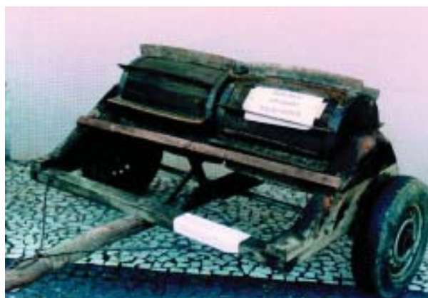
PLATE 79 Roller with blades with two cylinders and tyres
