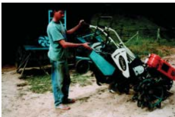
PLATE 57 Details of the disc and rotary hoe system which opens the furrow to place fertilizer as in the old models
