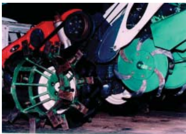
PLATE 57 Details of the disc and rotary hoe system which opens the furrow to place fertilizer as in the old models
