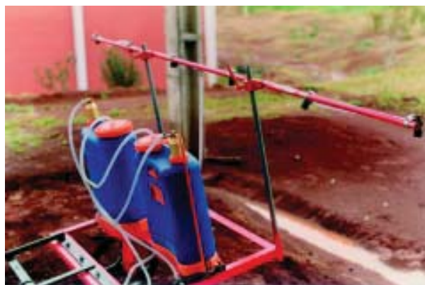
PLATE 86 Details of the spray bar, nozzles and tanks
