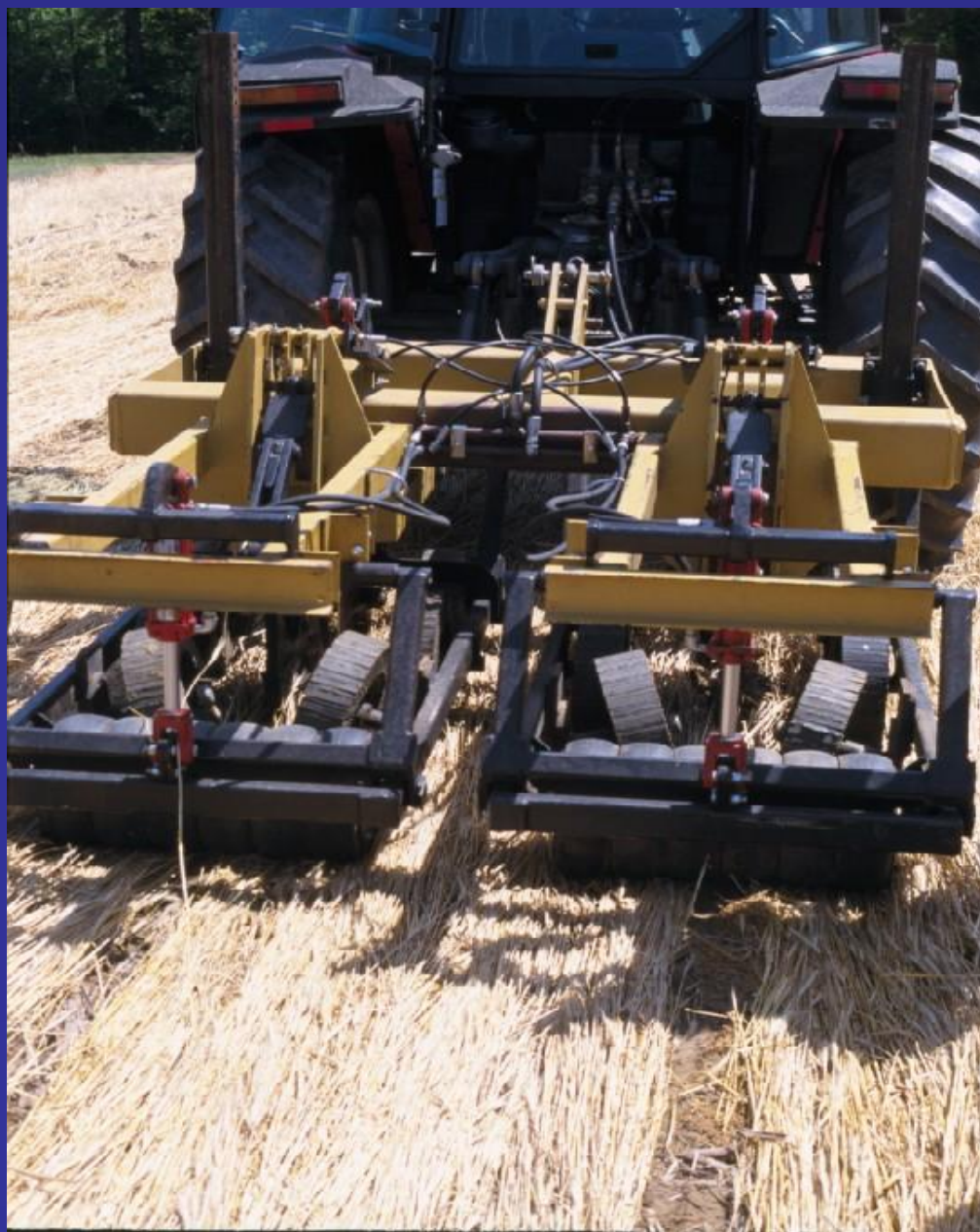
Non-inversion tillage can be integrated into high residue conservation systems. Shown here is a Precision Agricultural Tillage System (PATS) rig subsoiling in small grain residue after rolling. Note the minimal disturbance of surface residue.
