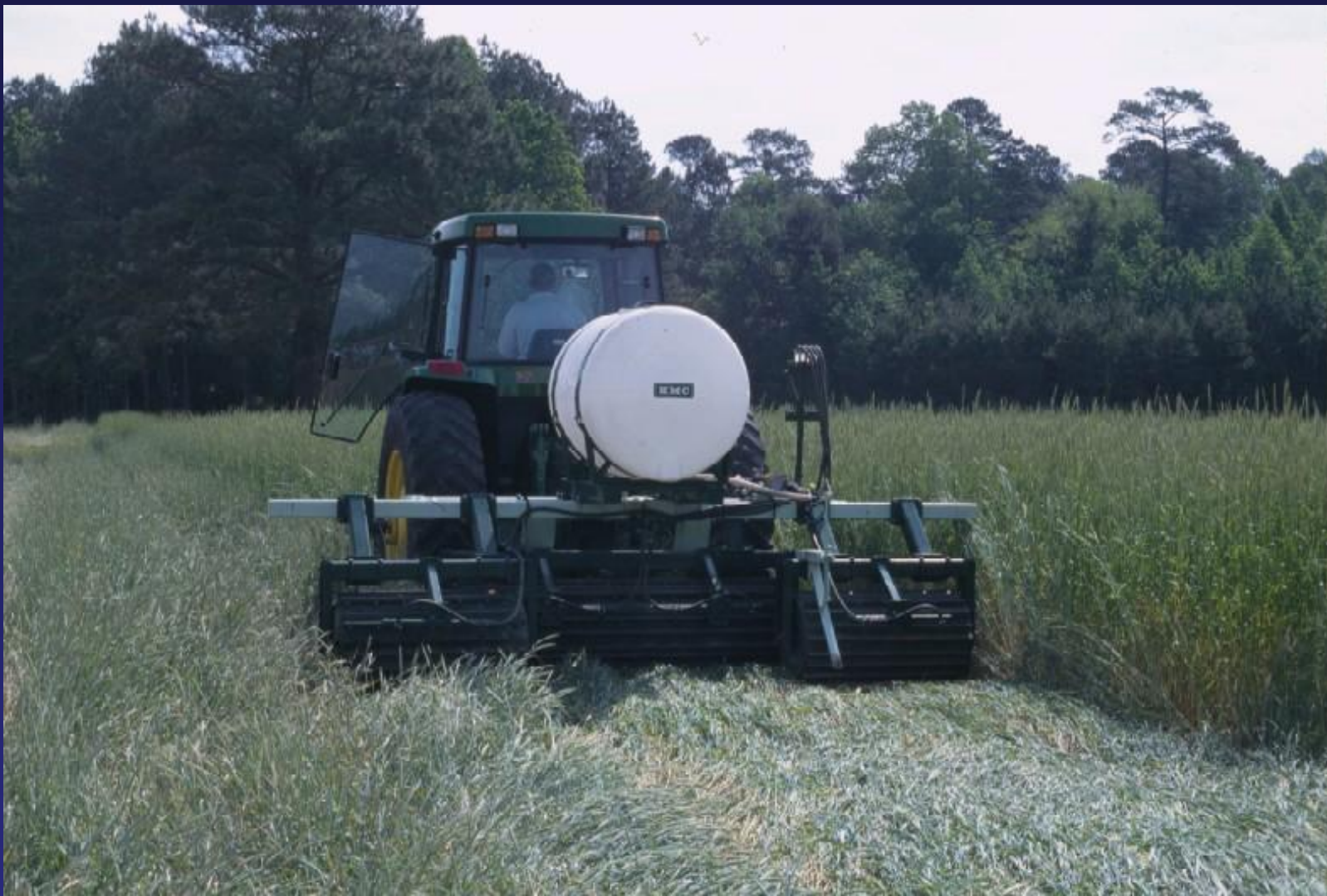
Mechanical roller-crimper manufactured by Kelley Manufacturing Company (KMC) of Tifton, GA. These units are inexpensive to build and operate. Roller may be front or rear mounted; front mounting allows for rolling, spraying, and planting in one pass.
