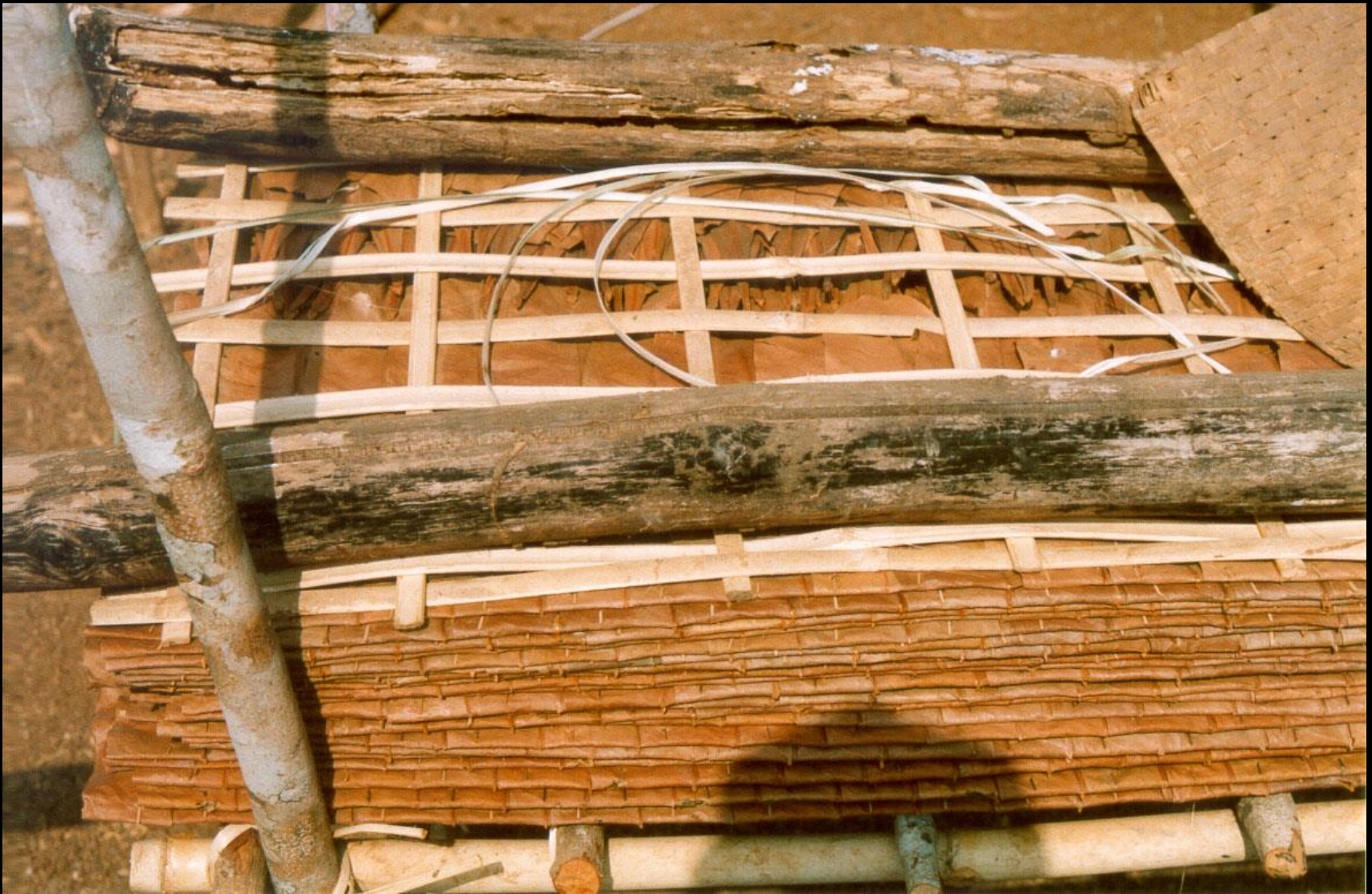
Roofing press. Forest leaves are pressed together in an interlocking mesh; the leaf bundle is held together using strips of thatch. After pressing, the finished “shingles” are ready to use.
