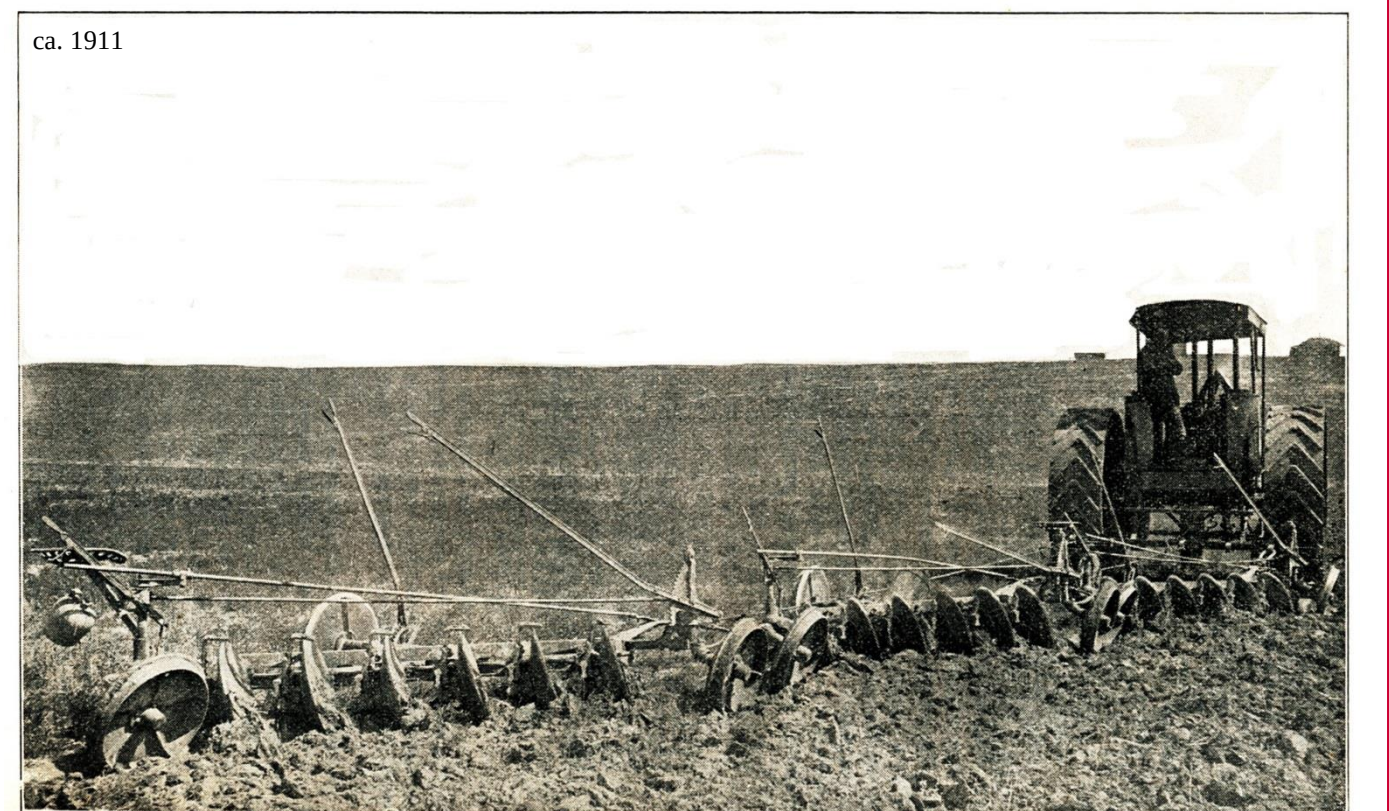
Plowing a Thomas county wheat field with a gasoline engine and three gangs of six plows each, cutting twelve feet.
