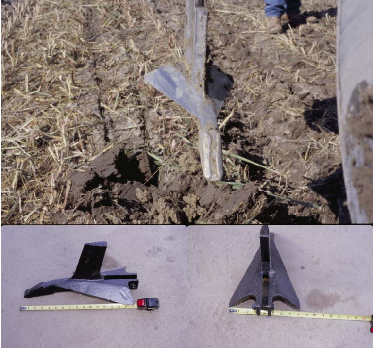
The TerraMax tool and its curved shank and point
