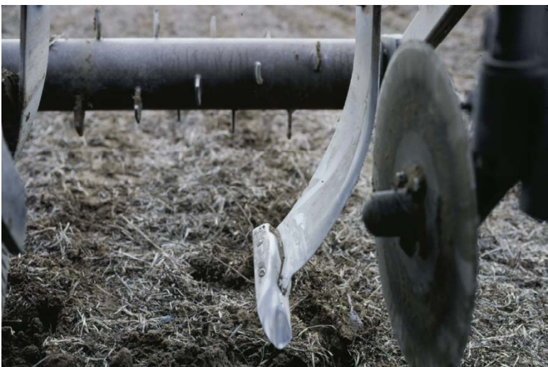
The TerraMax tool and its curved shank and point
