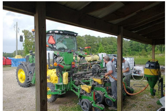
J John Deere 6110M tractor and precision planter used to plant corn and soybean plots. Randomized plot schedules are loaded into the tractor's computer providing positional guidance to the operator where to place the seed.
