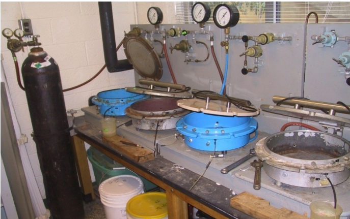
Figure 7.9.4 Pressure plate extractors for determining the soil water characteristic between -1,000 and -1,500 kPa. Normally, disturbed samples are tested in a pressure plate extractor. This is justified because water retained in the soil at high potentials is associated with the mineral matrix whose physical properties do not vary significantly.
