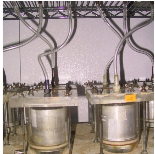
Figure 7.9.3 Tempe cells for determining the soil water characteristic between -10 and -100 kPa. Suction is applied to the soil column via supply tubing under controlled positive pressure. Water exits the column through a porous plate at the bottom until equilibration is reached. The applied pressure is assumed to be the matric potential of the column at that water content. Temperature must be controlled at all times during the procedure to minimize error from thermal dilation and contraction of water molecules.
