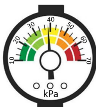
Figure 7.4.5 Left: thermometer measuring heat content in degrees Celsius with fill color indicating human comfort ranges. Right: dial gauge measuring water potential in kilopascals (kPa) with fill color indicating plant comfort ranges.
